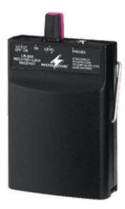
**Inductive receiver,** for receiving audio signals in inductive sound reproduction systems. The electromagnetic field which is created by an induction loop is received by the inductive receiver and converted into an audio signal. Any number of receivers can be operated within one induction loop.
